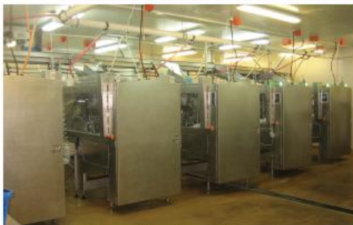
The production line at Sanford Havelock, with five automated mussel openers
