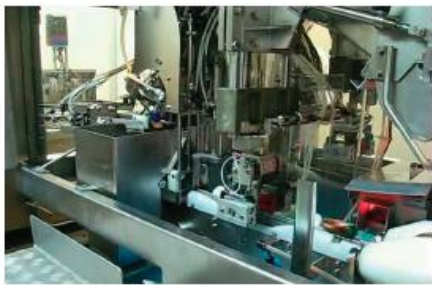
An automated mussel opener (above), and the technology that makes the operation possible (below), a scan picking up the physical orientation of a mussel as it is processed
