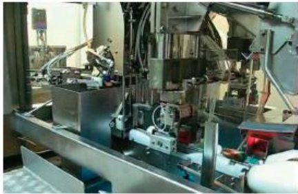
An automated mussel opener (above), and the technology that makes the operation possible (below), a scan picking up the physical orientation of a mussel as it is processed
